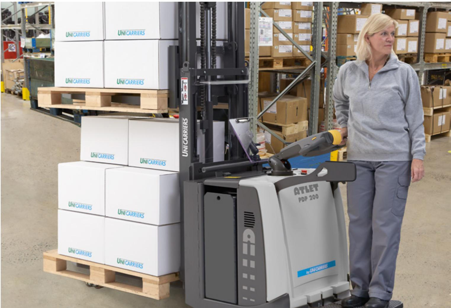
With a width less than that of a Euro-pallet, the PDP 200 has a total capacity of 2000 kg (1000 kg + 1000 kg in double pallet handling) and a maximum lifting height of 2090 mm. Its 2.2 kW AC-drive motor and driving speed of up to 12.5 km/h contribute to the unique pallet throughput of this efficient Double Stacker with ride on platforms (optional).
