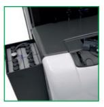
Low step in reduces fatigue and improves performance. An automatic floor sensor establishes driver presence and engages stop mode upon departure.
