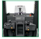
Pro-Access side gates with automatic sensors to prevent use of the truck with gates open when above 1200 mm.
